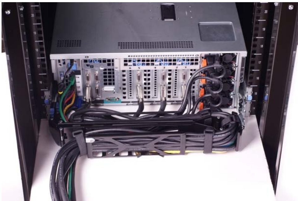
Figure 4: Left-Side Mounted CMA Installation
