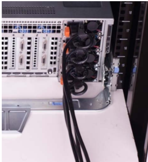
Figure 2: Routing Power Cables Through the Strain Reliefs
